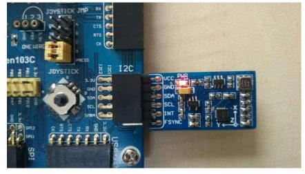
Figure 1: Connection between 10 DOF IMU Sensor (B) module and STM32
